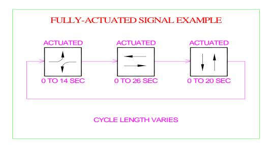
The maximum cycle length of 60 seconds for the above phasing scheme occurs when all phase sets are timed to their maximum value.
