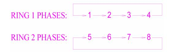
Common sense tells us that all phases on the main street must finish timing before any side street phase can receive the green and, conversely, that all side street phases must finish timing before any main street phase can receive the green. Going from the main street phases to the side street phases is called "crossing the barrier", as is the return from side street phasing to main street phasing. The barrier is the dividing line between main street and side street phasing.
