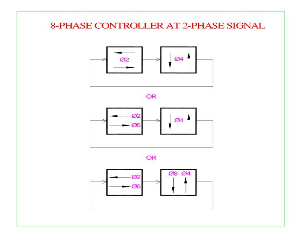
Quad operation is a phase rotation which utilizes all eight NEMA phases, having four left turn phases and four thru phases. The left turns on the main street operate concurrently with the opposing left turn and with the adjacent thru phase. The same operation occurs on the cross street. The term "quad" is used to describe this operation because there are four left turn phases (1, 3, 5 and 7):
