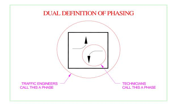
To maintain clarity, this course defines a **phase** as any traffic signal display with its own set of timings that controls an individual vehicle or pedestrian movement.
