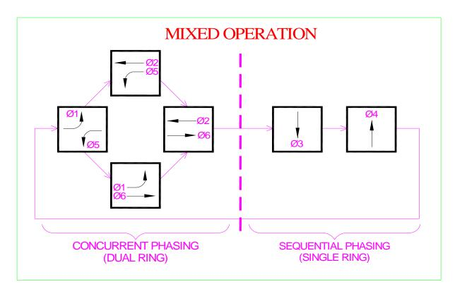
In this type of mixed operation, the dual ring phasing is typically found on the main street while the single ring phasing is usually found on the side street. An intersection with concurrent left turn phasing on the main street and split phasing on the side street is a good example of mixed operation.
