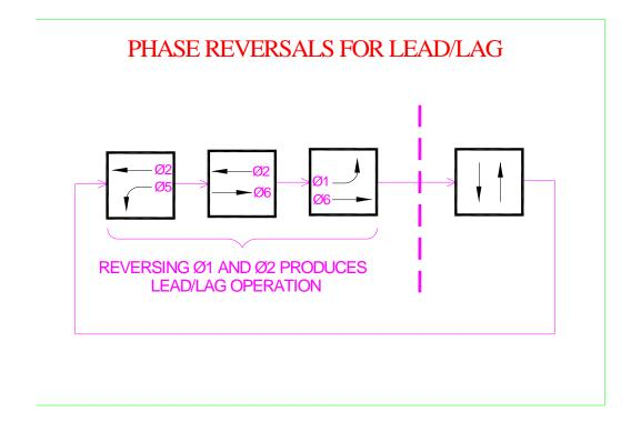
As their name suggests, when a phase reversal is active it switches (or reverses) the order in which two sequentially numbered phases are displayed within the phase rotation. For example, if a 1-2 phase reversal is active then phase 2 will precede phase 1 rather than following it, causing the phase 1 left turn to lag the phase 2 thru movement.
